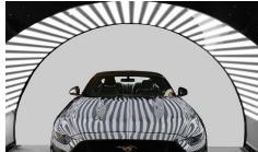
So-called "structured light" systems are critical in industrial inspection, e.g., to detect defects in car bodies [2]
