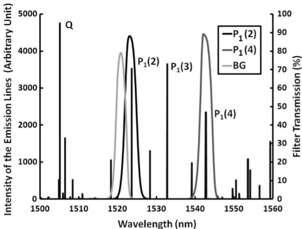
Figure 1: OH (3,1) Band. The gaussian lines are the filter's transmission
