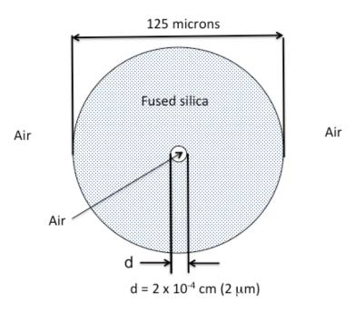
We want to fill the fiber with a mixture of two liquids that will allow it to propagate light in a single mode. The two liquids are carbon disulfide (CS<sub>2</sub>) with  $n_{1550nm} = 1.590$  and bromotrichloromethane (CBrCl<sub>3</sub>) with  $n_{1550nm} = 1.507$ . An approximate expression for the refractive index at  $\lambda_0$ =1550nm of a mixture that had X volume fraction CS<sub>2</sub> and (1-X) volume fraction CBrCl<sub>3</sub>, where 0 < X < 1, is given by
