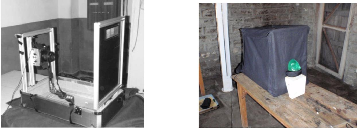
Fig. 2. Left: Prototype DR system showing x-ray screen on the right and Nikon D700 DSLR on the left. The frame folds down into the suitcase for transport. Right: Same system but with light-tight shroud in place. System is shown as set up in the Manang District Hospital, Chame, Nepal, with the breast phantom in position for imaging.
